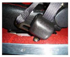
anos and others is the fact that they only use ONE of the tiny bolts in the roof to attach the belt. I just do not feel safe knowing that this ONE tiny 5/16" bolt holds the belt. The Morris kit, on the other hand, has a patented bracket. which attaches the seat belt to BOTH bolts in the roof...
